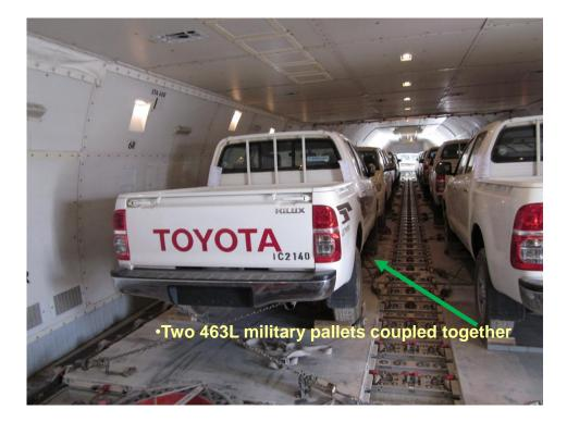
This Toyota Truck is on two 463L military pallets linked together by a coupler device in order to make one longer pallet. The military can link several of these together to make a "pallet train".
