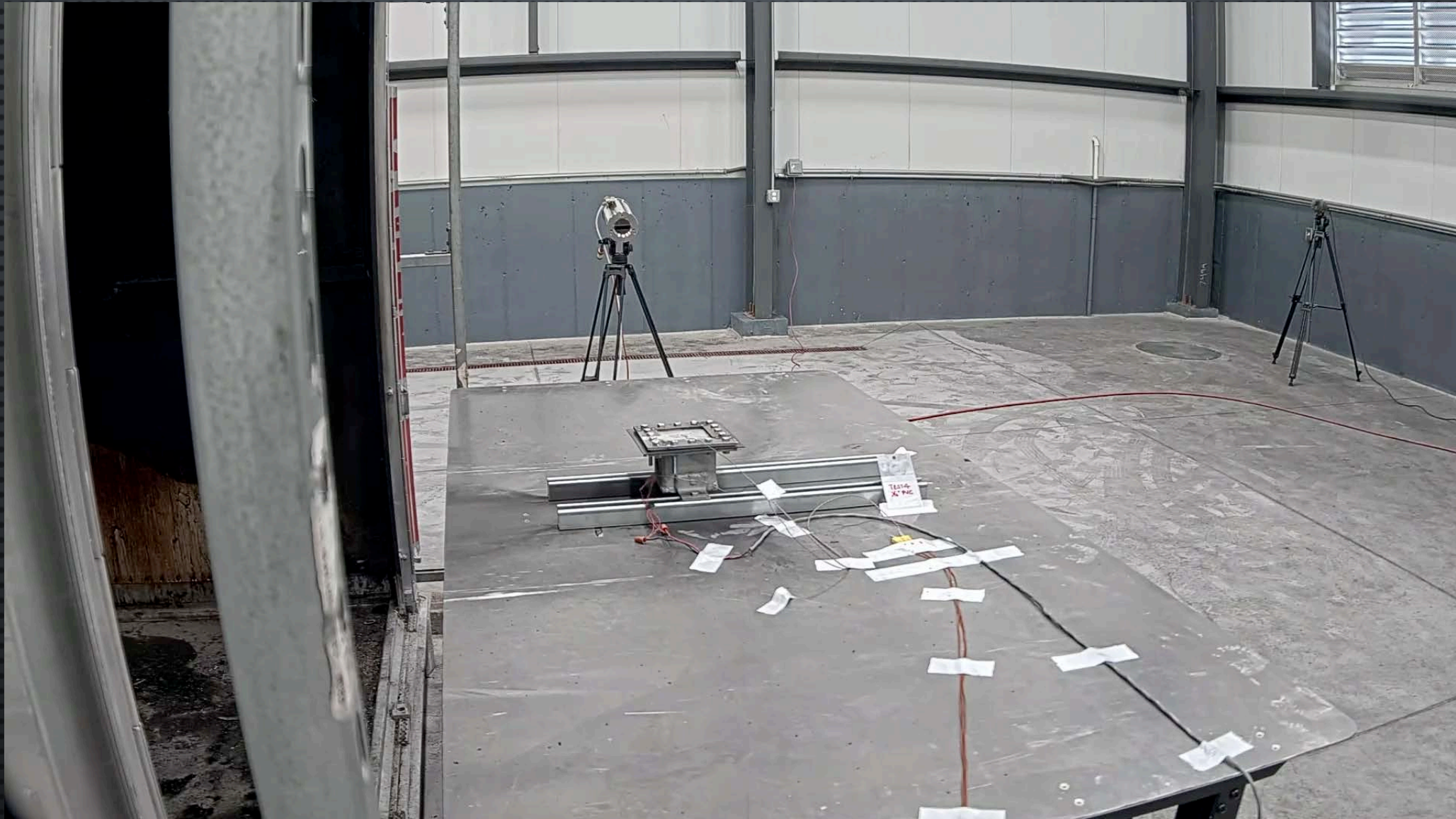
Baseline Test of a 3.3mm Al sample with 25x 18650 Lithium batteries
